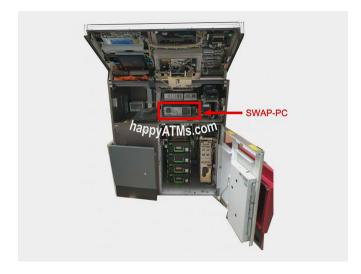
The computer within an ATM naturally plays a central role in the operation of the device. This computer connects to all the various critical components of the ATM such as the card reader, PIN pad, network interfaces, and ultimately, the cash cassettes.
