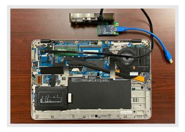
While the overall process was relatively straightforward, the attack **did require us to open the case of the device**. As noted earlier, such an open-chassis DMA attack would raise the risk from an attacker's perspective, but would still remain plausible for a dedicated adversary.
